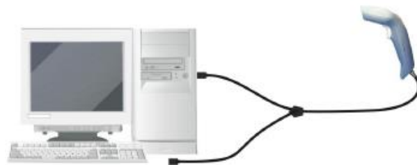
Figure 1: Connecting the reader to a PC
